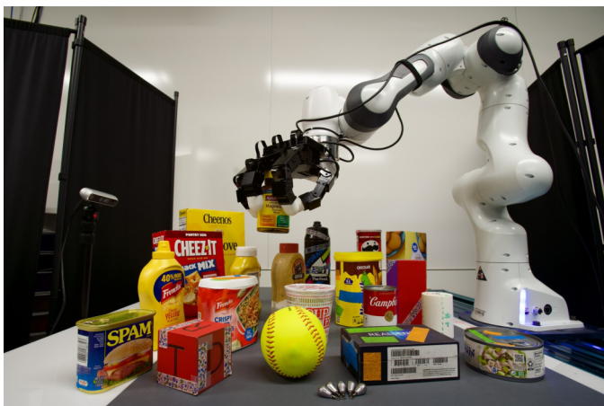
Fig. 4. Hardware setup for the dexterous manipulation experiments: a 7-DOF arm equipped with a 16-DOF dexterous hand, a camera for runtime perception, and household objects used for grasping and in-hand reorientation.
